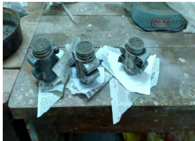
Fig.3 Performing U.C.S. sample specimen and mould
