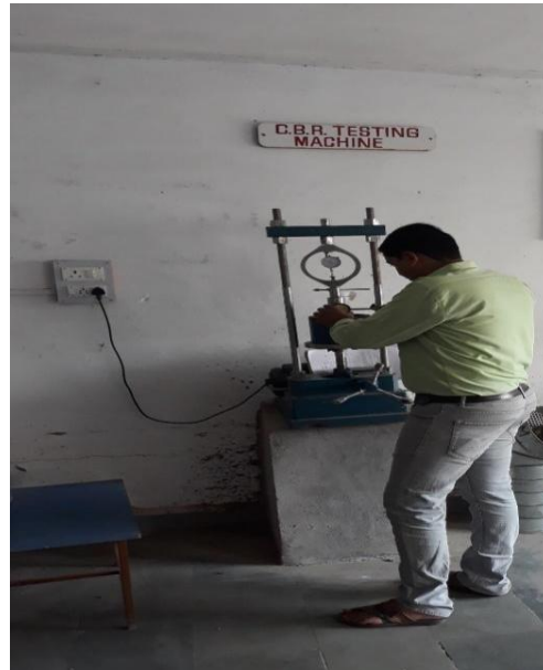
Fig.4 Performing Test of CBR soil specimen
