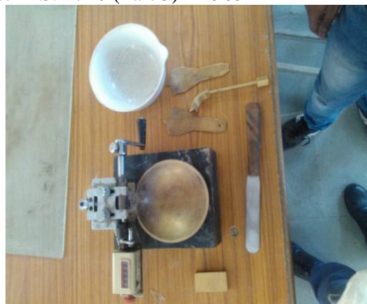
Fig.5 Liquid limit-apparatus & tools
