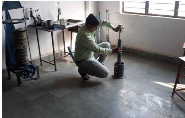
Fig.2 performing standard proctor test
