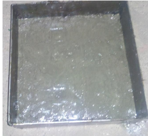
Casting of FRC + Concrete Block
