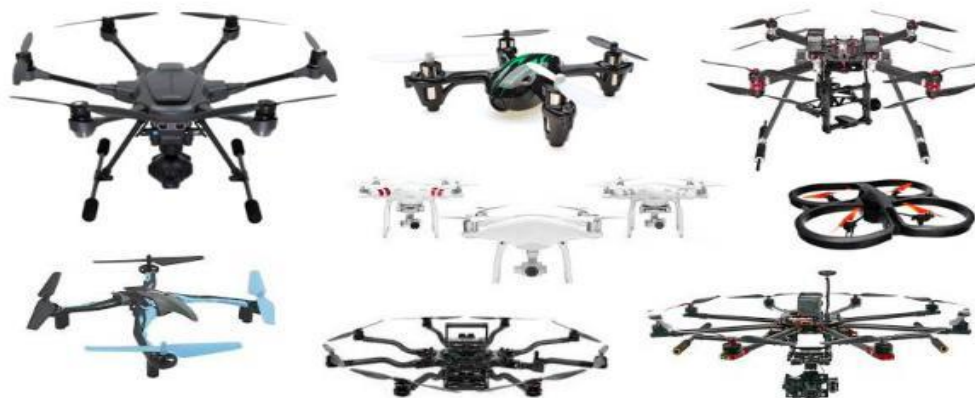
Figure: Multirotor drones: tricopter (3 rotors), quadcopter (4 rotors), hexacopter (6 rotors), and octocopter (8 rotors) (Source: https://www.aniwaa.com/guide/drones/drone-buying-guide/ )
