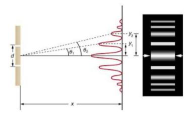
The interference pattern for a double slit has an intensity that falls off with angle. The photograph shows multiple bright and dark lines, or fringes, formed by light passing through a double slit.
