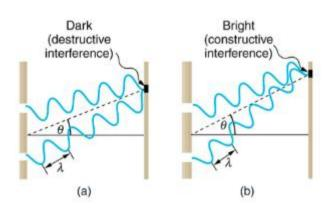
If the screen is a large distance away compared with the distance between the slits, then the angle between the path and a line from the slits to the screen (see the figure) is nearly the same for each path. The difference between the paths is shown in the figure; simple trigonometry shows it to be  $d \sin \theta$ , where is the distance between the slits. To obtain **constructive interference for a double slit**, the path length difference must be an integral multiple of the wavelength, or
