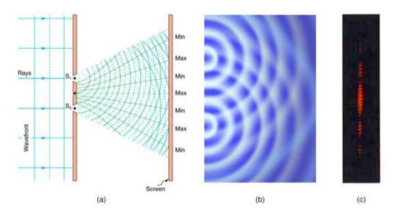
To understand the double slit interference pattern, we consider how two waves travel from the slits to the screen. Each slit is a different distance from a given point on the screen. Thus different numbers of wavelengths fit into each path. Waves start out from the slits in phase (crest to crest), but they may end up out of phase (crest to trough) at the screen if the paths differ in length by half a wavelength, interfering destructively as shown above in
