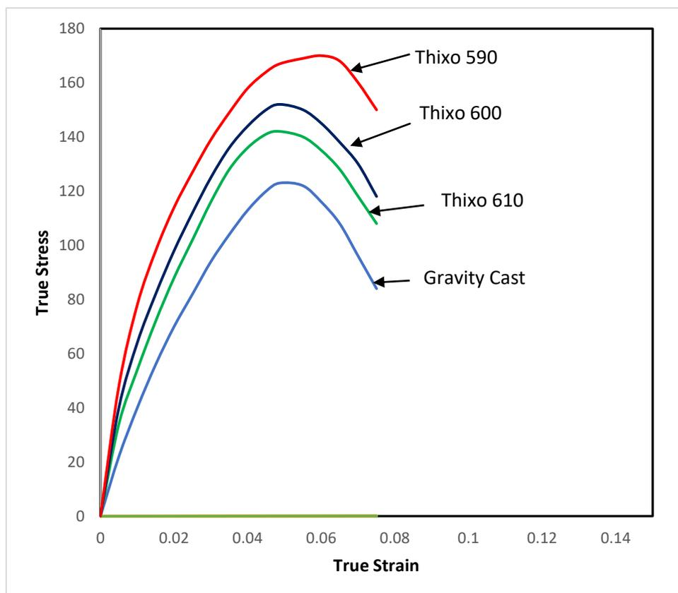
**Fig. 5 Stress Strain Curves**
