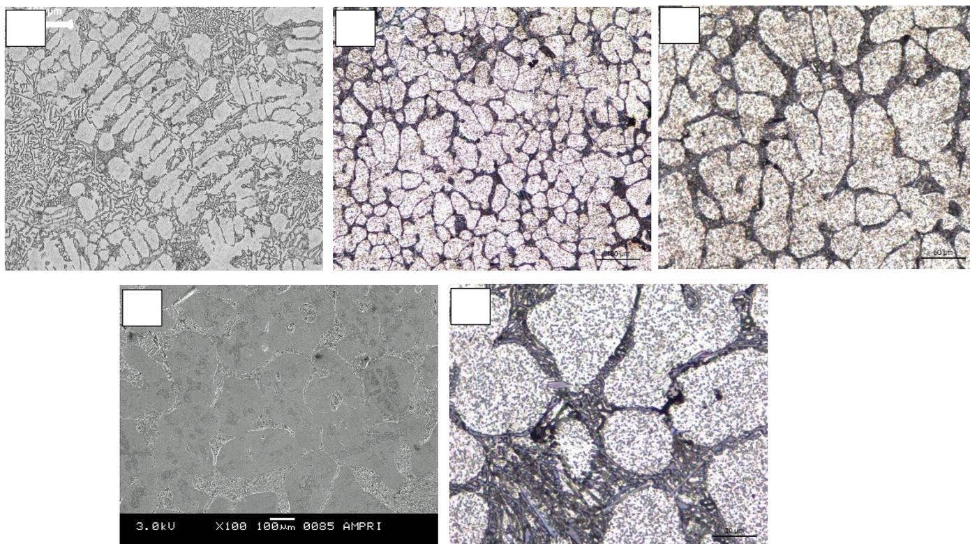
**Fig. 4 Microstructures - Gravity Cast and Thixocast LM25 Alloy: (a) Gravity Cast, (b) Thixocast at 590°C, (c) Thixocast at 600°C, (d) Thixocast at 610°C and (e) Nondendritic microstructure with finer  $\alpha$ -Al**
