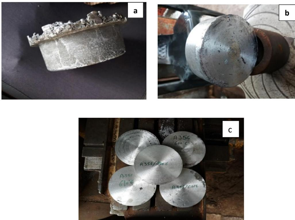
**Fig. 3 Thixocast Alloy (a) Before Machining, (b) After Machining & (c) After Machining ( at diff. processing temperatures)**
