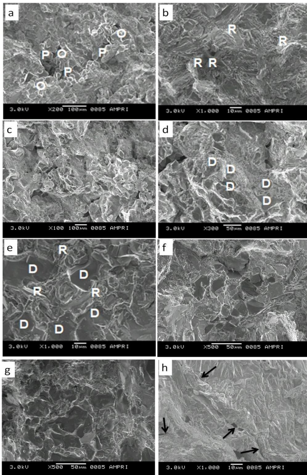
**Fig. 5 Fractographs : (a)&(b) Gravity Cast, (c)&(d) Thixocast at 590°C, (e)&(f) Thixocast at 600°C, (g)&(h) Thixocast at 610°C**
