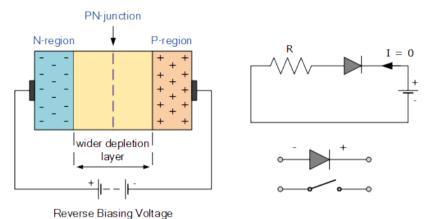
This condition represents a high resistance value to the PN junction and practically zero current flows through the junction diode with an increase in bias voltage. However, a very small **leakage current** does flow through the junction which can be measured in micro-amperes, (  $\mu$ A ).
