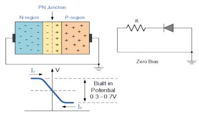
The potential barrier that now exists discourages the diffusion of any more majority carriers across the junction. However, the potential barrier helps minority carriers (few free electrons in the P-region and few holes in the N-region) to drift across the junction.
