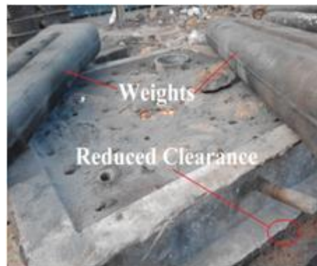
Fig.17. Heavy Weights on Cope
