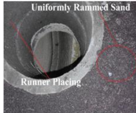
Fig.13. Sand Ramming and Runner Placing
