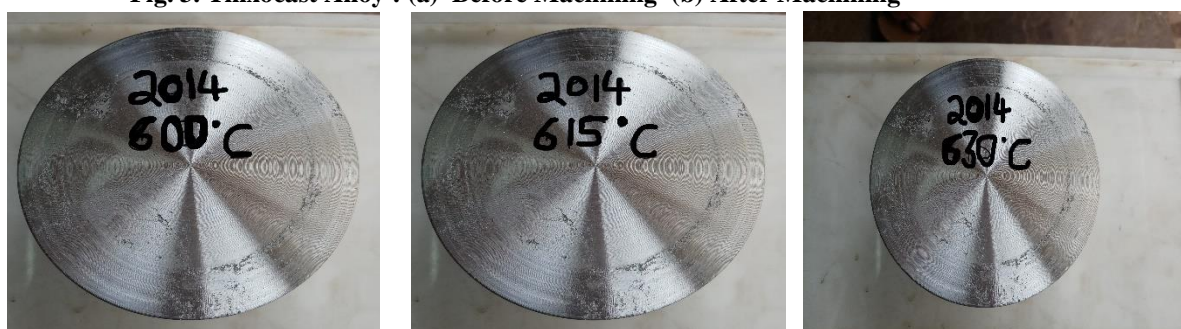
Fig. 3. Thixcast Alloy : (a) Before Machining (b) After Machining
