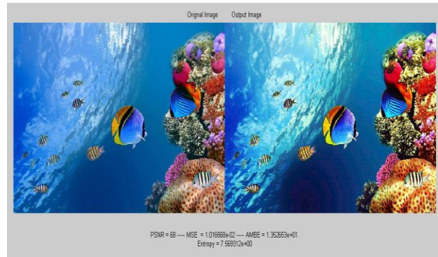
Fig.2 : Image of blue sea. Left image is original image and right image processed using Brightness Preserving Bi-Histogram Equalization Method
